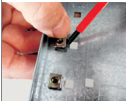
Insert the cage-nuts in the holes specifically for the device.
