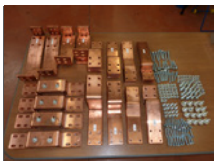
Connection kits for transfer supplied dismantled
